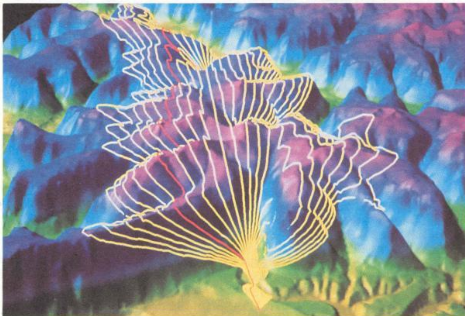
The map above displays a three-dimensional visualization of noise contours over terrain at Ft. Knox, using SG3d. Noise contours, depicted by the red, yellow, and white lines, were generated at five degree intervals between simulated sound source and listening points. Surface colors represent elevation, ranging from red at high elevations to yellow in the valleys. (graphic by Dave Gerdes, Bill Brown and Terry Baker, USACERL)
